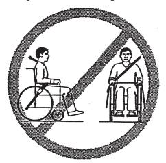
FIGURE 3 - FIGURES INDICATING IMPROPER POSITIONING OF OCCUPANT RESTRAINT(S)
